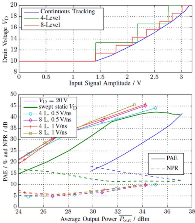
Fig.5. Trajectory for various types of tracking (top) and measured performance (bottom) for the MMIC PA from Fig.2. PAE and NPR are plotted as a function of average output power for a 100-MHz 11-dB PAPR signal.
