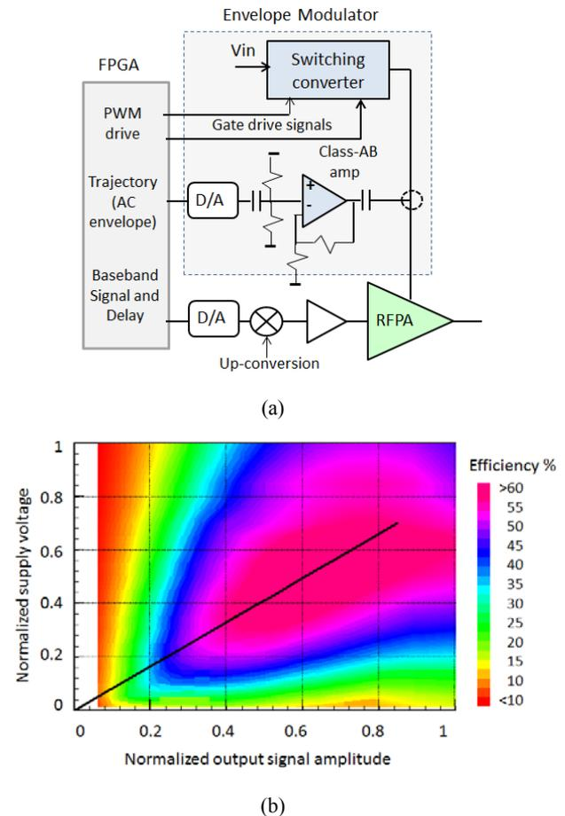
Fig.1. (a) Block diagram of a typical ET transmitter showing the high-efficiency RFPA, and supply modulator that consists of an efficient but slow switching dc-ed converter and a linear amplifier that provides the high-bandwidth signal component. (b) Typical dependence of efficiency on normalized supply voltage and output power of a PA.
