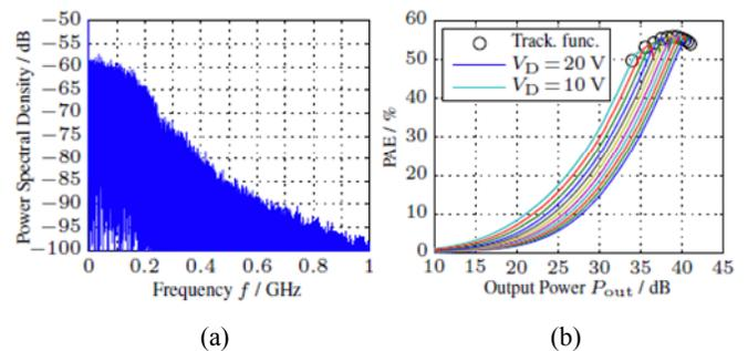
Fig.4. (a) Spectrum of a 250-MHz band-limited Gaussian noise signal that is continuously tracked. (b) MMIC PA from Fig.2 measured PA as a function of output power at 10GHz with points showing the tracking trajectory for constant gain.
