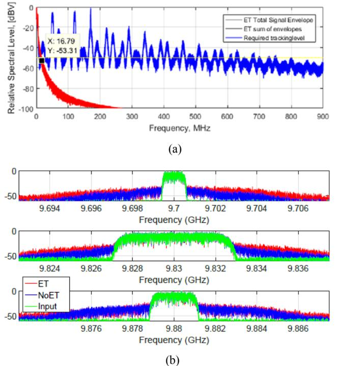
Fig.6. (a) Ideal spectra of combined envelope (blue) and summed envelopes (red). (b) Measured normalized individual signal spectra at the input of the PA (green), output of PA with no supply modulation (blue) and output of PA with reduced bandwidth supply modulation (red).
