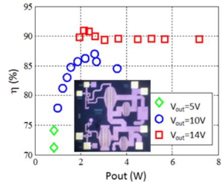
Fig.3. Measured efficiency of a 100-MHz switching GaN MMIC Buck converter (2mm square) for three dc voltages. The efficiency includes the low- and high-side drivers.
